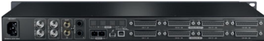
The Orion 32+ Gen 3 is the latest offering from Antelope Audio. Housed in a sleek 1U rack-mount, the unit offers an amazing 64 simultaneous audio inputs and outputs. 32 analogue I/O is on the rear panel, with the remaining connectivity via various digital connections. However, that is not all, the Orion 32+ Gen 3 also sports stereo monitor outputs on TRS additional to the 32 analogue outs.
