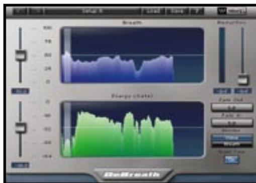
above are met, the breath sound is faded out of the voice path and into the breath path. The timing of this fade is user-defined, as is the reverse — i.e. when the signal is faded from the breath path and back into the voice path. Similarly, the amount of movement of the signal is also variable, so that some breath noise remains in the voice path, but is attenuated by a certain level.
