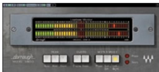
case of 'poacher turned gamekeeper', Dorrough designed a new 'loudness meter' combining the best features of PPM and VU with improvements to ballistics made possible by LED displays and microprocessors.
