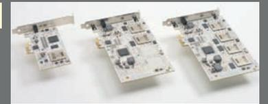
Solo, Duo or Quad UAD-2 cards can be mixed or matched in any combination of up to four cards. Each UAD-2 is powered by single and multi-chip configurations and offers 2.5x (Solo), 5x (Duo) and 10x (Quad) the power of a UAD-1.
