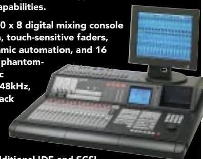
Good use is made of internally-illuminated keys and eight rotary encoders, four with a concentric ring of LEDs, for EQ gain, frequency, Q and pan. These can be paged to address the aux sends of the selected channel. Rotary encoder 'gearing' is selectable between 'coarse' and '1 step'. I found coarse too coarse and 1 step too fine for my liking.
