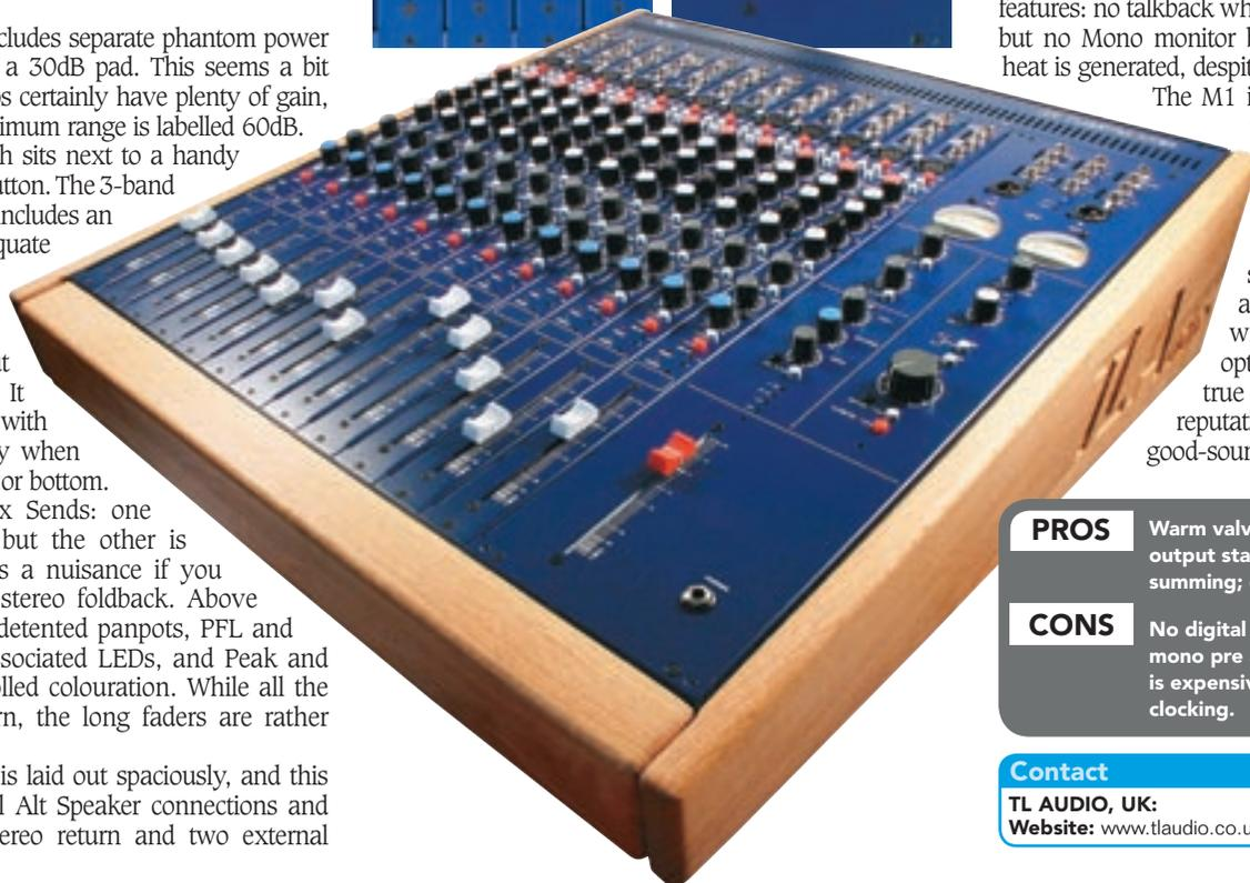
selectable 2-track monitor inputs, a PFL Balance knob, separate headphone level control, and a wonderfully huge Volume knob. A couple of illuminated circular VUs stylishly indicate mix level.
