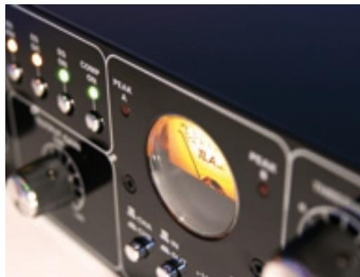
peak LEDs illuminate if things start to get out of hand — typically when THD levels reach 10%. In use, this tube stage is really very useful, acting gradually on a signal and warming it up gently for the first three-quarters of its travel, and then much more overtly in the last quarter. But even when cranked up quite high it manages to avoid sounding overly 'gritty' as some other units can tend to.
