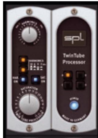
I duplicated and balanced tracks in order to compare processed and unprocessed signal, as there is the glaring omission of any kind of level trim to counter the boost that happens (up to 6dB) from turning up the Saturation. The Harmonics control enriches the high frequencies at one of four selectable frequencies from 2kHz to 10kHz. In the hardware version a
