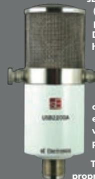
The USB2200a employs proprietary chips. One transforms the 5V power supplied via the USB cable to power the capsule after first removing noise and spikes from the current. A second chip includes the appropriate software drivers for plug-and-play use with any DAW.
