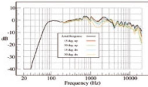
Fig. 3. Vertical off-axis response.
