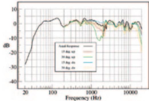
Fig. 3. Vertical off-axis response.
