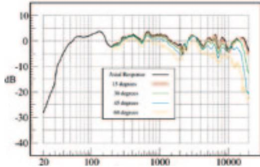
Fig. 2. Horizontal off-axis response.
