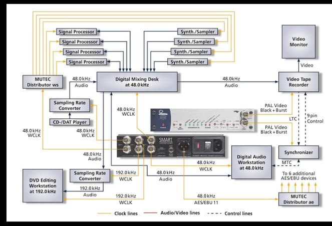
application shows that all video and audio devices, as well as a synchroniser, receive their reference clocks phase-locked in a similar manner from the Smart Clock AV.
