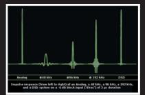
of self-noise. Fifth order noise shaping is used to shift this out of audible range. Analogue filtering is minimised and no decimation is needed in the digital to analogue conversion. SACD is capable of 120dB dynamic range with a 100kHz frequency response.
