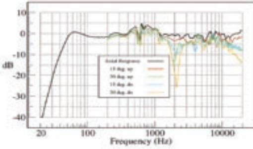
Fig. 3. Vertical off-Axis Response.
