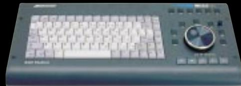
A precision, optically-encoded jog wheel with a concentric shuttle ring allows control of audio or video with frame accuracy.
