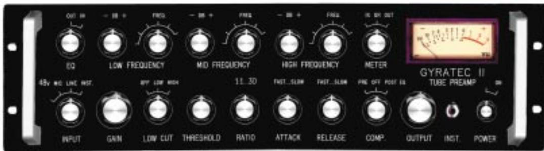
**I**N RECENT YEARS, the Danes have taken their audio very seriously, and this Gyraf is no exception. It is an all-tube recording channel with a mic/line preamp, EQ and compressor. Solid state components feature only in the sidechain and power supply, the signal flow only passes through valves, transformers and passive components.
