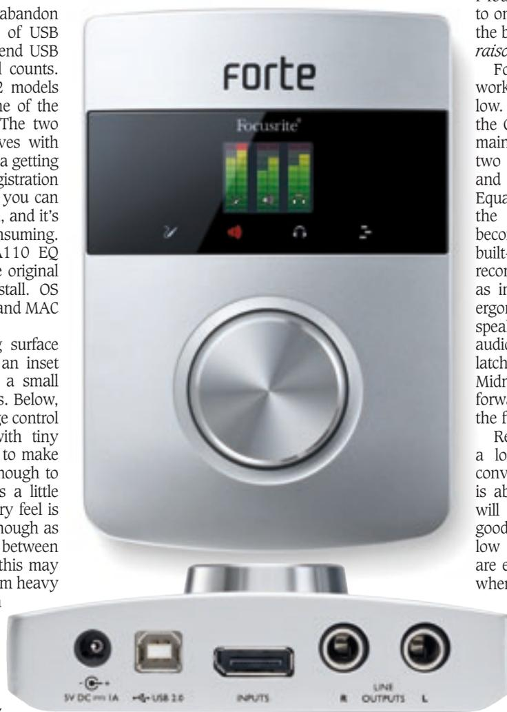
has made good use of the space available to display relevant information and to make menu navigation as easy as possible. The mode icons — Input, Main Output, Headphones and DAW — have modes of their own. A short touch selects the mode and a longer one opens the relevant menu. For inputs and outputs a second short touch toggles between channels.
