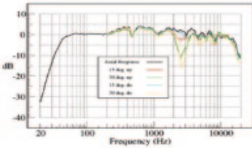
Fig. 3. Vertical off-axis response.
