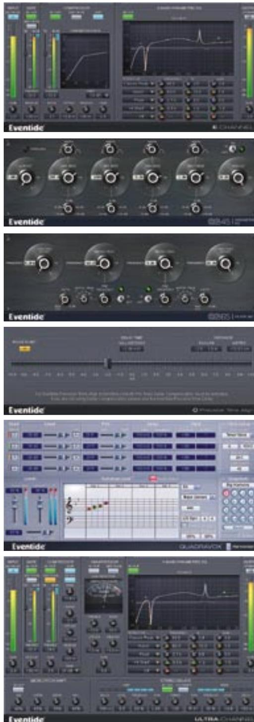
High and Low Cut filters, but featuring a pair of extremely narrow Notch/Peak filters, each with six modes: 5%, 10% and 50% of centre frequency for Notch or Peak. This is an unusual and useful tool for problem solving, and both EQs sound remarkably analogue, thanks to 48-bit double precision filters.
