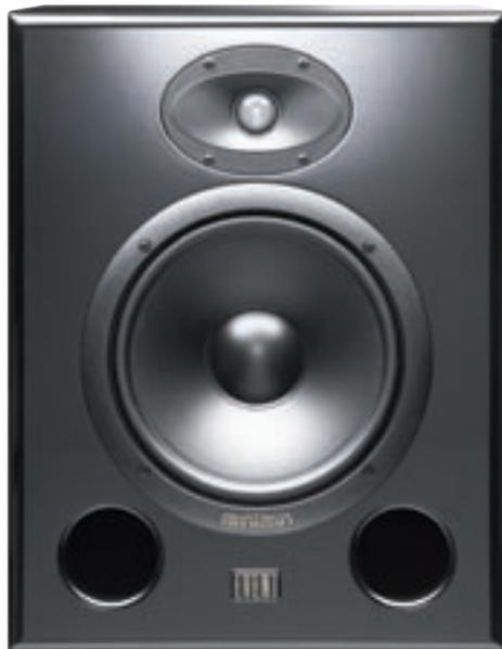
The Event Electronics Studio Precision ASP8 is a two-way active loudspeaker consisting of an 8-inch (200mm) mid-bass driver with a mineral-filled polypropylene cone, and a 1-inch (25mm) soft-dome tweeter that radiates through a shallow, elliptical horn-type waveguide. Both drivers have neodymium magnets and are magnetically-shielded. The drivers are mounted in a vertical orientation on the front baffle of a
