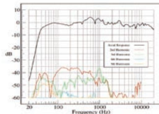
Fig. 1. On-Axis Frequency Response and Harmonic Distortion.
