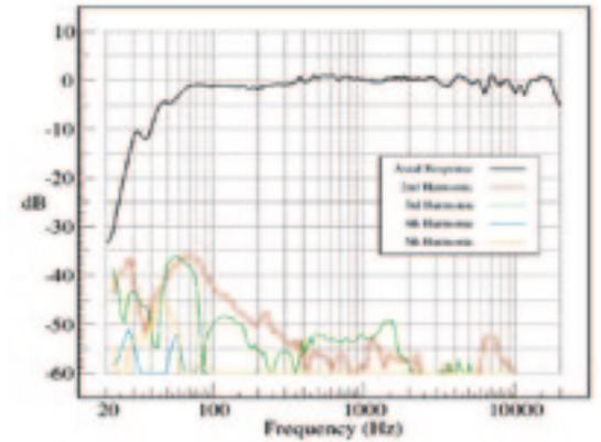
**Fig. 1. On-axis frequency response and harmonic distortion.**
