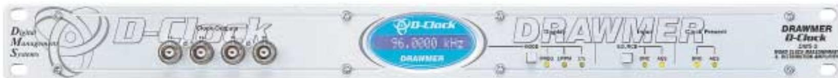
**A**LTHOUGH IT IS POSSIBLE to make do with just a few Word clock outputs from the master source, looping them through several devices, this is undesirable and a source of potential problems with clock phase and terminations. A star arrangement, with each device fed from a separate socket, ideally with equal length cables is the preferred configuration. However, in a complex studio, this can mean a lot of outputs.
