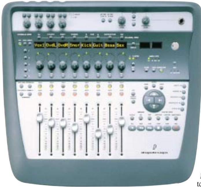
**WHILE THE (STILL CURRENT) DIGI 001** is a PCI audio and MIDI interface, the 002 uses Firewire to connect to the host computer. The package looked at includes Pro Tools 5.3.2 for Mac OS 9.2.2 or Windows XP, and the 002 will work with iMacs, Apple Laptops and Sony Vaio laptops, although desktop PCs need a Firewire card.
