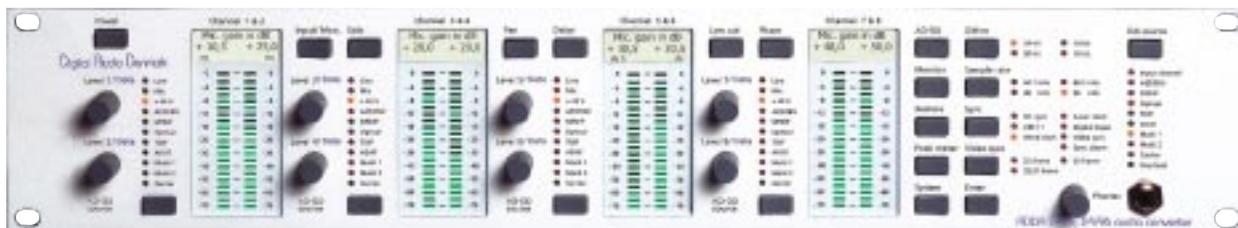
through a number of options for each input channel that can be set using the relevant data entry knob, regardless of the type of input selected. These options are a switchable high pass filter (80Hz), phase reverse and a variable delay of up to 100ms on each channel. Each of these parameters can be viewed or altered for each of the eight channels by pressing and holding dedicated 'short-cut' buttons located along the top of the unit.
