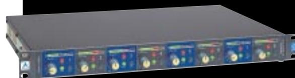
line in/line out transformer-coupled line amplifiers in a single 1U rackmount. Variable gain controls are provided and permit output levels to be trimmed to different levels from the same source when used as a distribution amplifier, or enable different input levels to be trimmed to provide equal output levels from each of the eight channels. A 'Silk' switch introduces a circuit that is said to emulate the sound of classic Rupert Neve designs.
