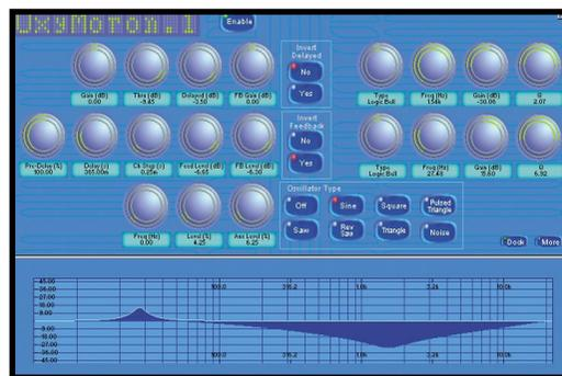
underlying Cue (audio recording) for the duration of the Event (EDL entry) with the effect applied and replaces the original in the Event list. The original Event remains in the list but is 'Stated Out' i.e. muted. Thus allowing for quick comparisons and instant undo even on machines without any plug-ins.
