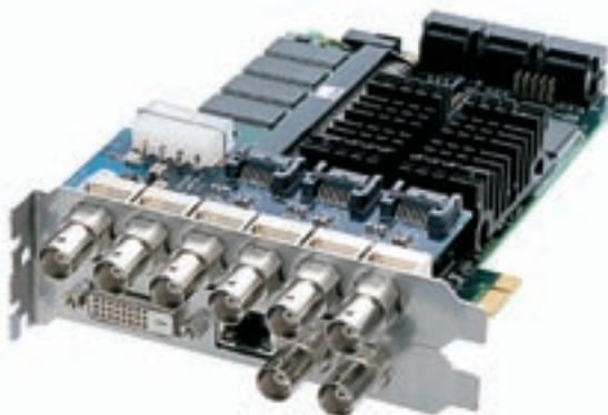
The Crystal architecture is based on the use of high-density FPGAs. Each of these chips contain millions of simple logic parts, that can either statically or dynamically upload a program that configures those parts into complex arrangements for high-speed computer applications. These applications will be used to replace media signal processing hardware that was previously composed of dedicated components or partially-programmable digital hardware.
