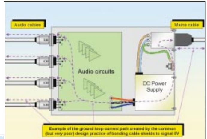
Example of the ground loop current path created by the common (but very poor) design practice of bonding cable shields to signal 0V
