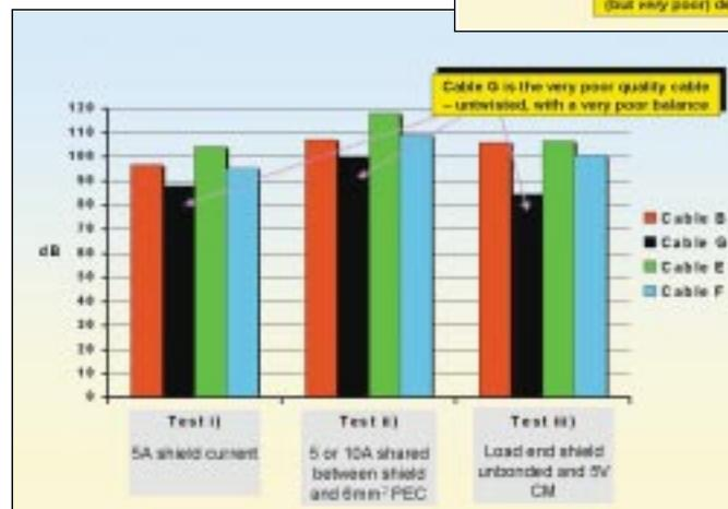
**Figure 2. Cable CMRRs for a floating 75 ohm source**
