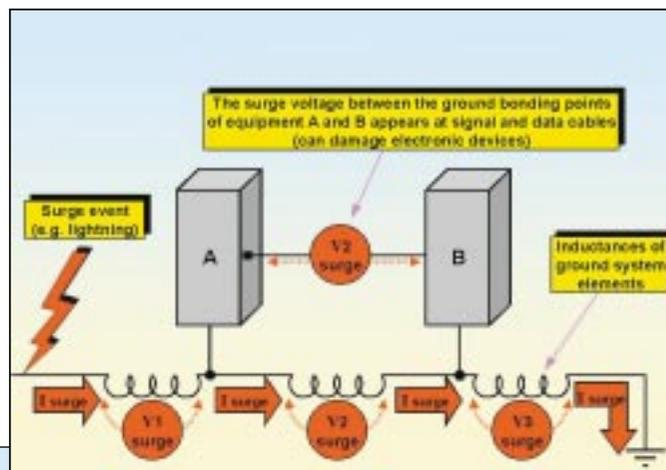
Figure 5. Surge overvoltages caused at signal inputs and outputs
