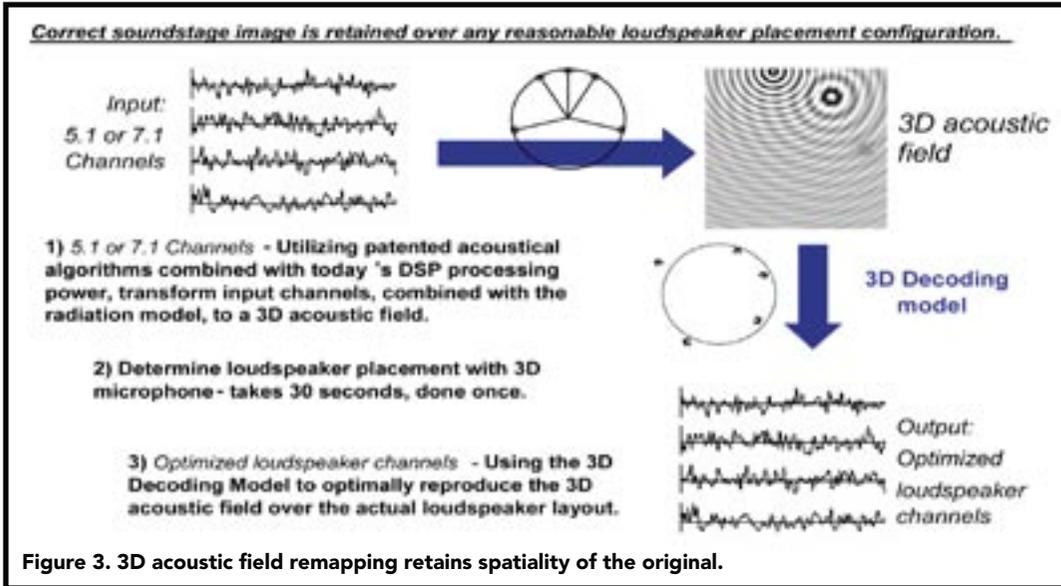
Figure 3. 3D acoustic field remapping retains spatiality of the original.
