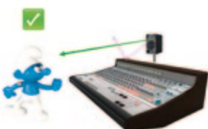
Figure 3. Console reflection minimised by relocating loudspeaker.
