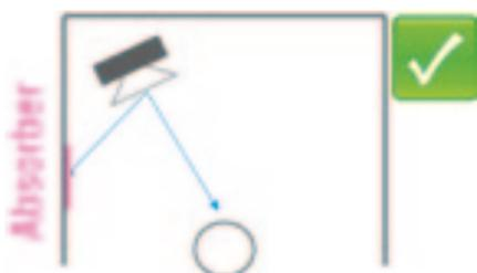
Figure 5. Side wall reflection minimised by absorption.
