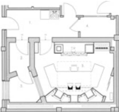
Figure 8. KIFF Aarau, Switzerland; side wall reflection minimised by room geometry.
