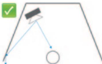
Figure 7. Side wall reflection minimised by room geometry.
