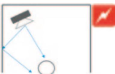
Figure 4. Side wall reflection interfering with direct sound.
