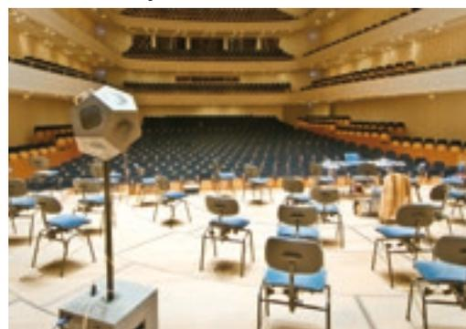
Figure 3. Omnidirectional measurement loudspeaker, KKL Luzern Concert Hall.
