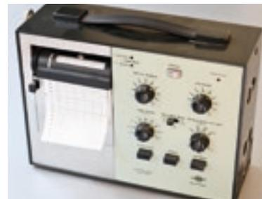
Figure 2. Plotting device (Bruel & Kjaer 2317 Level Recorder).
