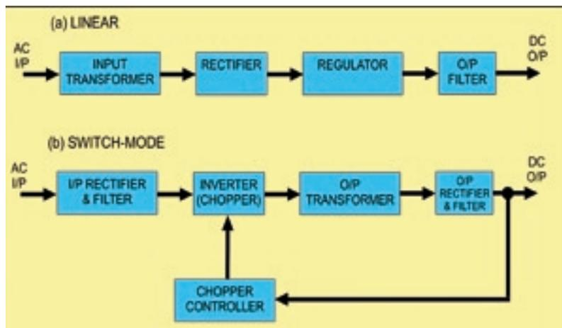
**Figure 1. Basic block diagrams of linear and switch-mode supplies.**
