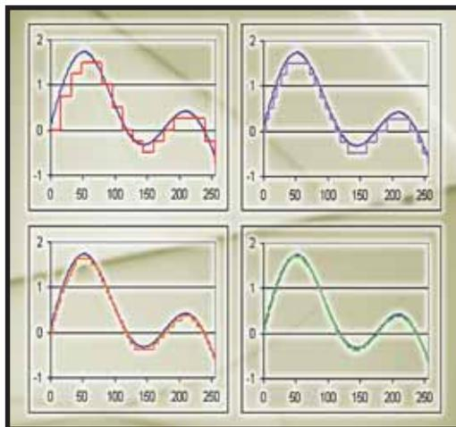
The top-left figure shows the original signal and the result of a (bad) analogue to digital conversion. In the top-right figure, the sampling frequency has been doubled but the resolution is kept unchanged. The result, even though not perfect, better matches the analogue signal. The sampling rate of the bottom-left figure is the same as the one of the top-right figure but the resolution has been doubled. Again it's an improvement.
