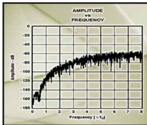
In the presence of high frequency noise, the semiconductors are subject to a phenomenon called 'input stage RFI rectification'. While amplifying small signals in the audio band, these devices can rectify unwanted high frequency signals. This results in DC error, which appears at the output in addition to the wanted signal.
