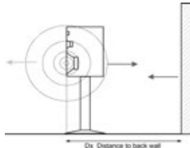
**Wall behind the loudspeaker cancellation phenomenon. Distance to wall =  $\frac{1}{4}$  wavelength.** (Courtesy of Genelec)
