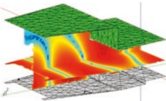
**Acoustic Boundary Element Calculator (ABEC) model — low frequency analysis of a listening room. The red areas represent high pressure zones while blue areas indicate low pressure zones.**
