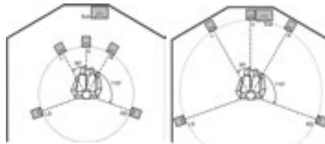
**ITU-R BS.775-1 loudspeaker placement with satellite speakers placed at least 1.1m from the wall and placed against a hard wall (Hemispherical loading).** (Courtesy of Genelec).
