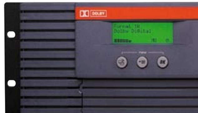
latter have always been the biggest offenders in terms of high sustained levels. So as part of the installation for a commercials and trailers agreement is a Dolby loudness equivalent meter known as an Leq meter.
