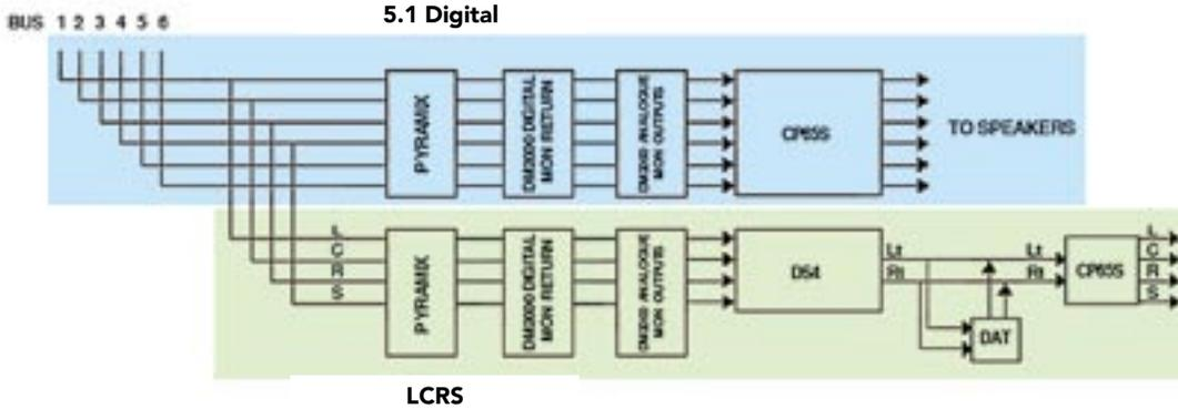
or predictable. Hence, whereas with 5.1 there is no need to have an encode/decode system while you're mixing, with LCRS you need to monitor through the entire chain to hear what you're doing. To this end Dolby provides on loan, free of charge to every certified studio, a DS4 encoder; this also means that Dolby can take it back at any point should your standards drop too far.
