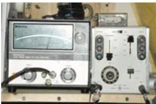
Good audio-certified voltmeters do not have to cost a lot. Here's a picture from my test bench of another classic, a Ballantine True RMS AC Voltmeter I bought surplus for US\$35, attached to a Hewlett Packard attenuator/balanced bridge I picked up for \$10. It can measure signals from 300 volts down to the noise floor in microvolts.
